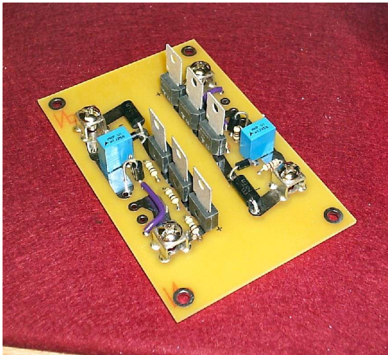
Figure 17. Actual SISG board less IGBTs.
